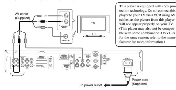
1. Connect the VIDEO OUTPUT and AUDIO OUTPUT FRONT/D.MIX 1 jacks to a set of AV inputs on your TV.
